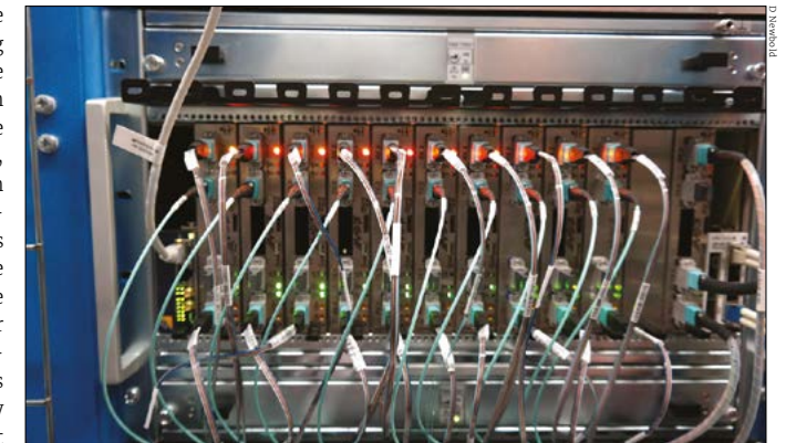
Workhorse Nine calorimeter-trigger cards process CMS events in parallel, while a 10th receives their outputs. The 11th is spare. Each card has a Xilinx Virtex 7 FPGA (pictured on p29). The cards were installed at the beginning of LHC Run 2 and will be upgraded for high-luminosity running.
