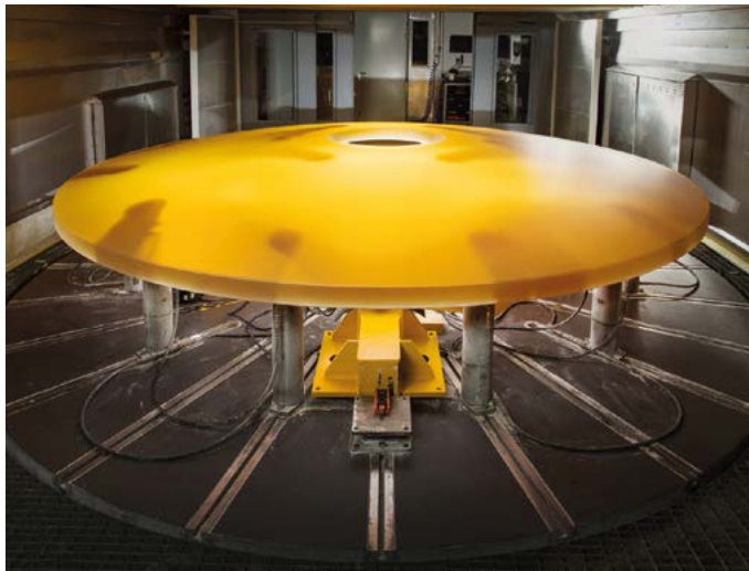
Ahead of the curve Top: architectural concept drawing of the 80 m-high ELT at work. Bottom: the three-tonne "blank" for the ELT's secondary mirror, machined from a slab of the low-expansion ceramic ZERODUR, in January 2019.
