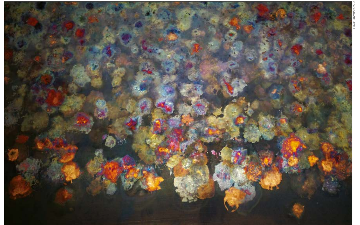
Flourishing physics The interior of a radio-frequency cavity used in a cyclotron at the GANIL (Grand Accélérateur National d'Ions Lourds) facility of the CEA and CNRS, showing regions that have been pulverised by the high-voltage electric arcs.
